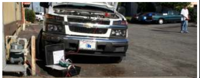
TRUCK BATTERY USED TO POWER OSCILLATOR
